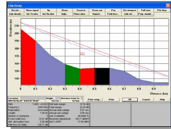
Link analysis showing terrain profile and detailed link information
