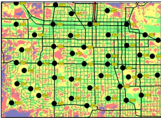
Complete coverage map that has optimized transmitter deployment locations
